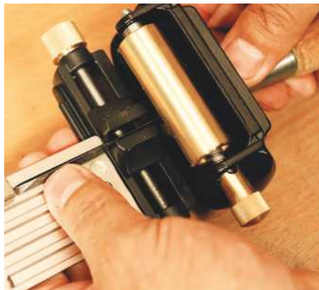
▲ The chisel or iron is slid up against the stop...
